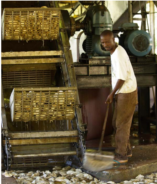
This spread, clockwise: The raw cup rubber is washed of impurities; then granulated to a popcorn-like consistency in preparation for being flattened into sheets; next it is moulded and baked into bales of a deep golden colour that are trimmed to weigh 35kg; the bales are wrapped and loaded onto pallets ready for export
